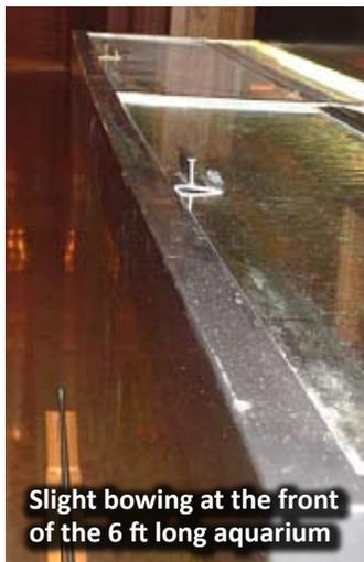
I posted on our forum looking for suggestions on what course of action to take and how to proceed. Some suggested using a chemical cement glue to attach piece of acrylic to either the top brace and frame, or to the front and back glass to prevent any further bowing out of the glass. Others suggested replacing the aquarium with a new one.
